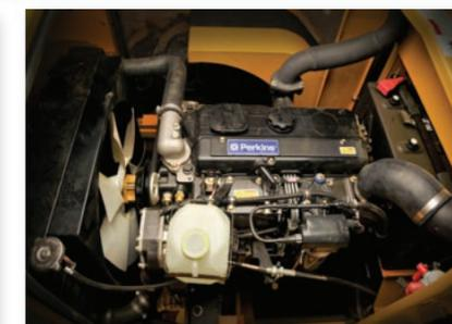
**ENGINE:** The P Series forklifts have a sliding hood for easy access during maintenance, and house a Perkins Turbo Tier 3 emissions compliant diesel engine.
